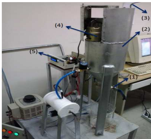
Fig 1 System of paddy soaking (1: water valve, 2: Tank, 3: Basket, 5: Agitator and 6: System of temperature control)
