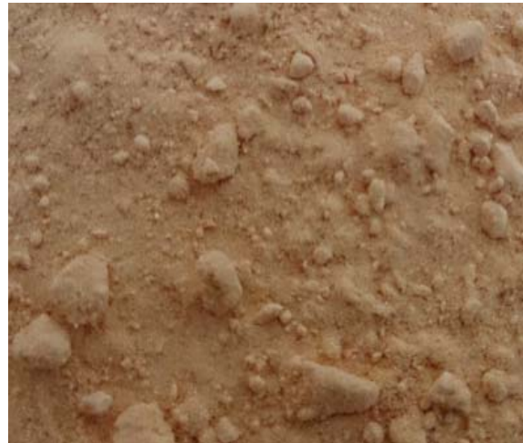
Fig 2 Powder samples produced in the presence of 40% MD and 5% DS in 150°C inlet air temperature
