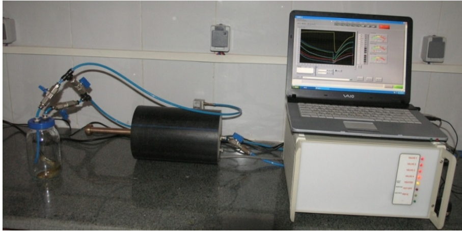
Fig 1 Schematic of electronic nose instrument made of carrier gas (1), flow meter (2), valve (3), odor sampling vessel (4), sensors chamber (5), data conditioning & acquisition interface (6), data acquisition and analysis soft wares (7).
